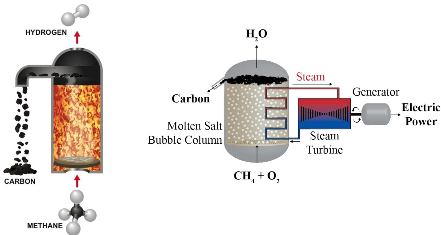
"Using a liquid catalyst allows you to overcome these challenges when used in a bubble column. The less dense solid byproducts float to the surface and then can be skimmed off, so the catalyst doesn't deactivate and it doesn't plug up the reactor," says Upham.
