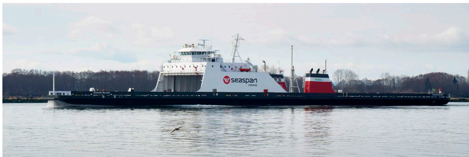
Figure 1. Seaspan Ferry that uses natural gas for propulsion
